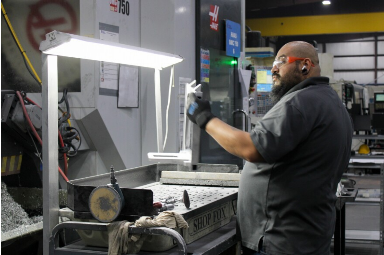
Jose Lopez, a machinist at Etezazi Industries, uses a hand grinder to smooth the edges on an aircraft part.
